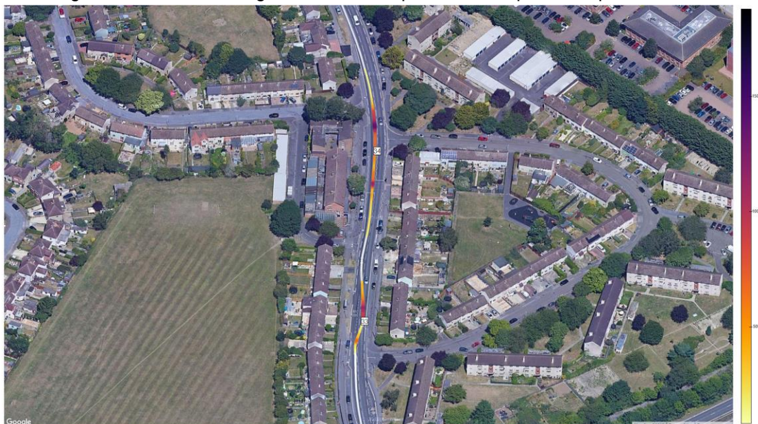
Figure 4: NO x levels produced by the Euro VI bus negotiating parked cars and congestion
