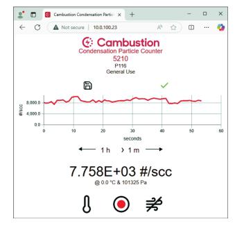
The 5210 supports control over Ethernet, USB or RS232, with open protocol commands to automate your own experiments. All protocols are documented in the manual.
