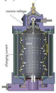
the touchscreen, or measured by the optional Aerosol Flowmeter accessory (see below). The user can specify a constant ion concentration - time product (n<sub>i</sub>t), the charger will calculate and supply the optimum charging current for the given sample flow, temperature and pressure.
