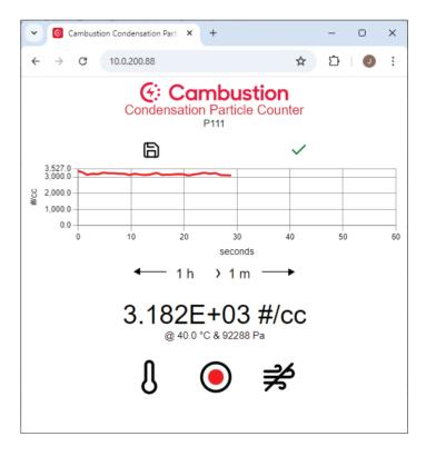
The 5210 supports control over Ethernet, USB or RS232, with open protocol commands to automate your own experiments.
