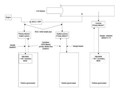
Figure 2: Recommended DPF sampling configurations, pre- and post-DPF and in CVS dilution tunnel
