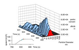
Figure 1: Particulate spectrum downstream of DPF measured with the DMS500: accumulation mode breakthrough occurs at high space velocity during high speed acceleration.
