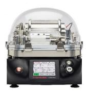
The CPMA is used with an external pre-charger, which may be of the radioactive, X-ray or corona types.
