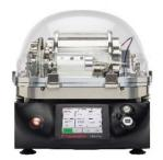
The CPMA is used with an external pre-charger, which may be of the radioactive, X-ray or corona types.
