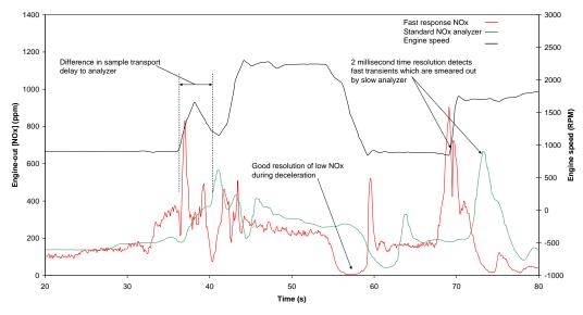
The figure above shows a typical portion of this highly transient cycle. The 3-4 second delay in the standard analyser is not uncommon and can easily be adjusted for by data manipulation. However, the 1,000 x faster T10-90% response time of the CLD500 does have an advantage when resolving the rapid transients; the red trace in the plot above reveals some high frequency information which is smoothed-out within the green trace.
