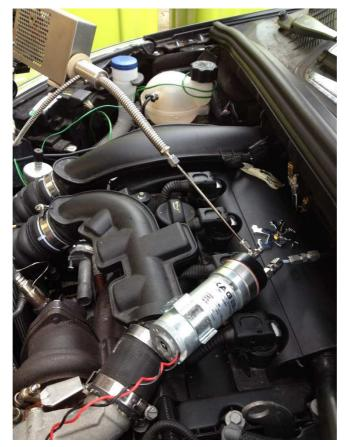
A solution is to use a small volume pump to extract just enough sample gas from the intake manifold to satisfy the flow requirements of the fast FID and then use the fast FID to sample from the pump's exhaust. By sourcing a pump which runs hot enough to avoid any significant liquid HC hang-up, but with small enough trapped volume to avoid slowing down the resulting response time too much, a system has been designed which yields a T10-90% response time of less than 100 milliseconds.
