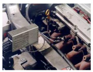
Figure 1: HFR500 sampling head and probe in exhaust port
