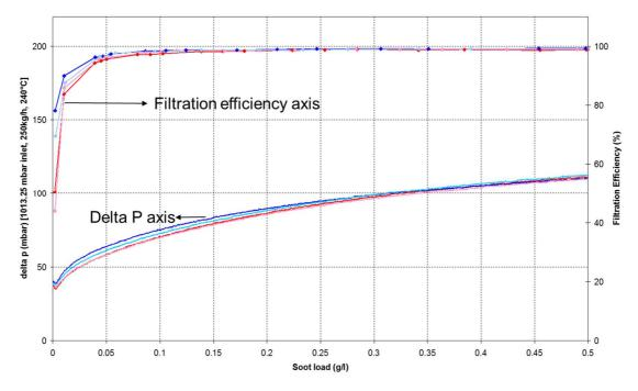
Figure 1: The back pressure and filtration efficiency results from two coated GPFs showing repeats as light colours.
