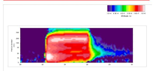
The size spectra were automatically volume weighted and assumed unit density to provide instantaneous and integrated mass.
