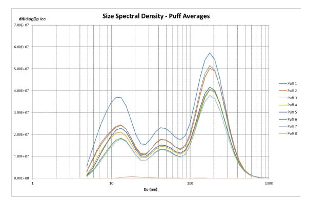
There is greater variability observed in this test, compared with the automatically triggered e-cigarette previously tested in application note 12. The short interval between puffs means that the device will not have cooled to equilibrium conditions between puffs, and indeed there is a systematic trend observed in the mass concentration.
