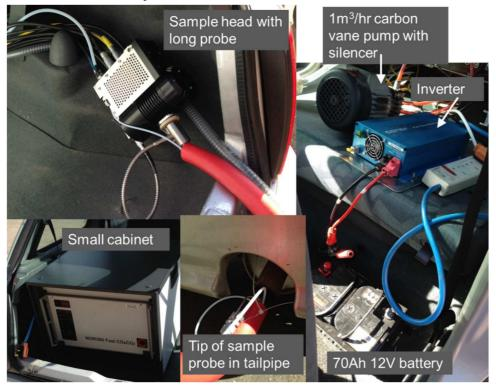
*Important user note:* avoid fitting probe tip too far into exhaust tailpipe and sampling water from muffler. Vacuum pump exhaust pipe should be routed to outside to avoid toxic gases entering the vehicle.
